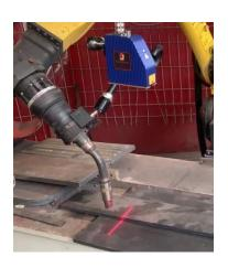
Before welding, the sensor takes 2 or 3 measurements on the weld seam on the workpiece to determine position and direction. The correcting signal is send to the robot controller and the robot corrects the original programmed position and locates the weld torch on the starting point of the weld seam. The weld process then acts according to the robot program.
